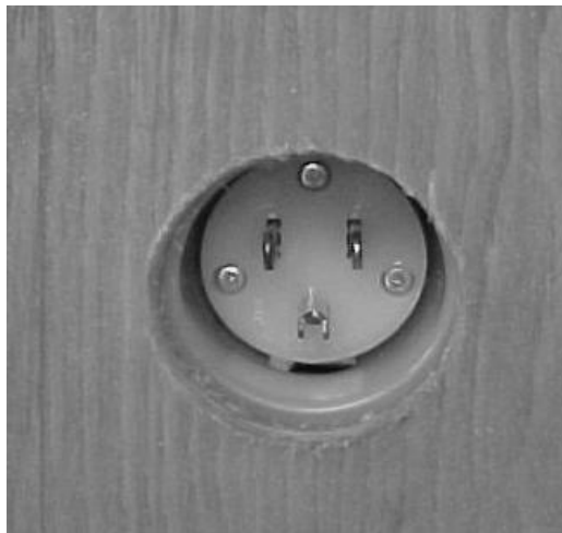
This is the outside of the kiln showing the 120 volt male plug.
